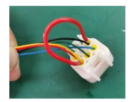
3- Power on the controller, if the indicator light no longer flashes 13 times at this time (no flashing or the flashing times is not 13 times), it means the controller is no problem, there is something wrong with the motor.
